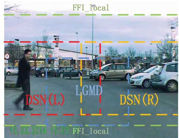
Fig. 2. A deployment of the separated field of view of the proposed system. The area enclosed by a blue box is connected to the LGMD subsystem while in the red and yellow box, DSNs (L) and DSNs (R) are deployed respectively. A FFI neuron captures the outputs of whole field photoreceptor cells and two extra regions at the top and bottom of the field vision are connected to a FFI_local component for distinguishing between moving and stop of vehicles.
