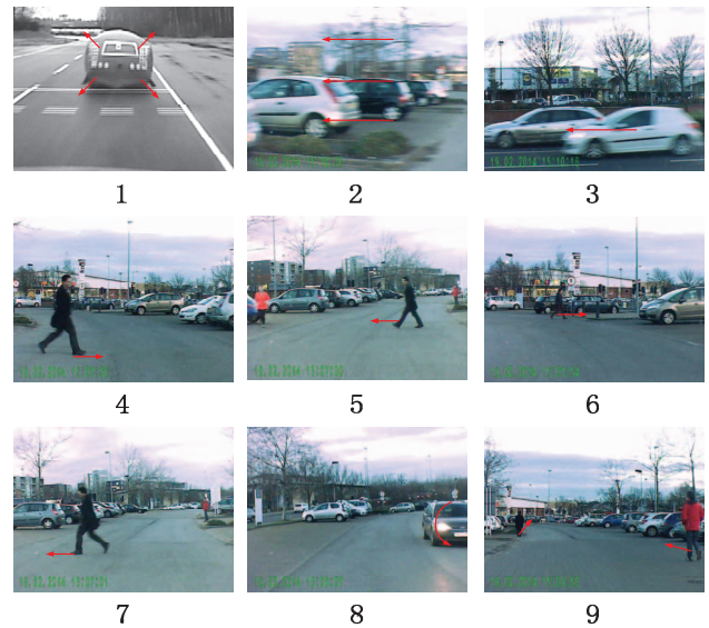
Fig. 3. Samples from video sequences represent driving environments. The car with the camera is moving forward at different speeds in all the above sequences but sequence 3. The arrows in the images are added to indicate visual motion directions. Video sequence 1 is a car collision scene at about 45mph; video sequence 2 is a left-turning scene at low speed (about 10 mph, the same to the rest if not state differently); video sequence 3, the car with camera with no movements while other cars passing from right to left; video sequence 4 is a left walking pedestrian from the left side of road to the centre; video sequence 5 is a right walking pedestrian from the right side of road to the centre; video sequence 6 is also a left walking pedestrian from the left side of road, but he is far away from the camera; video sequence 7 is a pedestrian walking from the centre of the road to the left side; video sequence 8 is a car driving in the right lane from distance; video sequence 9 is some pedestrians walking along the both sides of the road. Among the test videos, sequence 1, 4 and 5 are dangerous as they are developing quickly to imminent collision and need to trigger alarm. Sequence 2 is a difficult scene. For the proposed system, the FFI neuron will suppress the output of the LGMD subsystem and give a signal representing the global turning.
